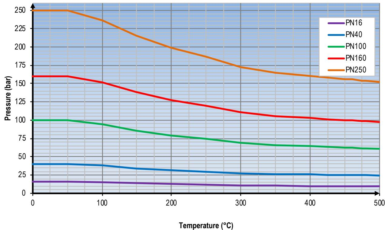
Forged stainless steel A182 F316L - according to EN1759-1
