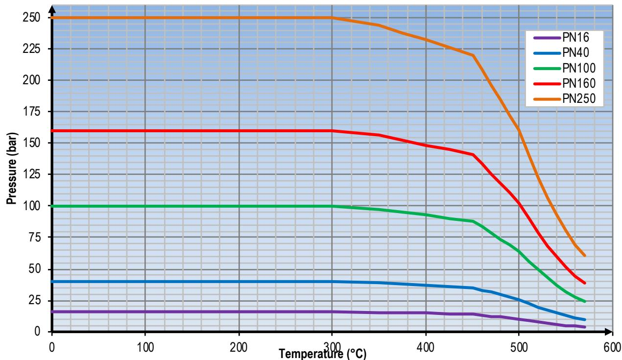
High temperature forged stainless steel A182 F22cl3 - according to EN1759-1
